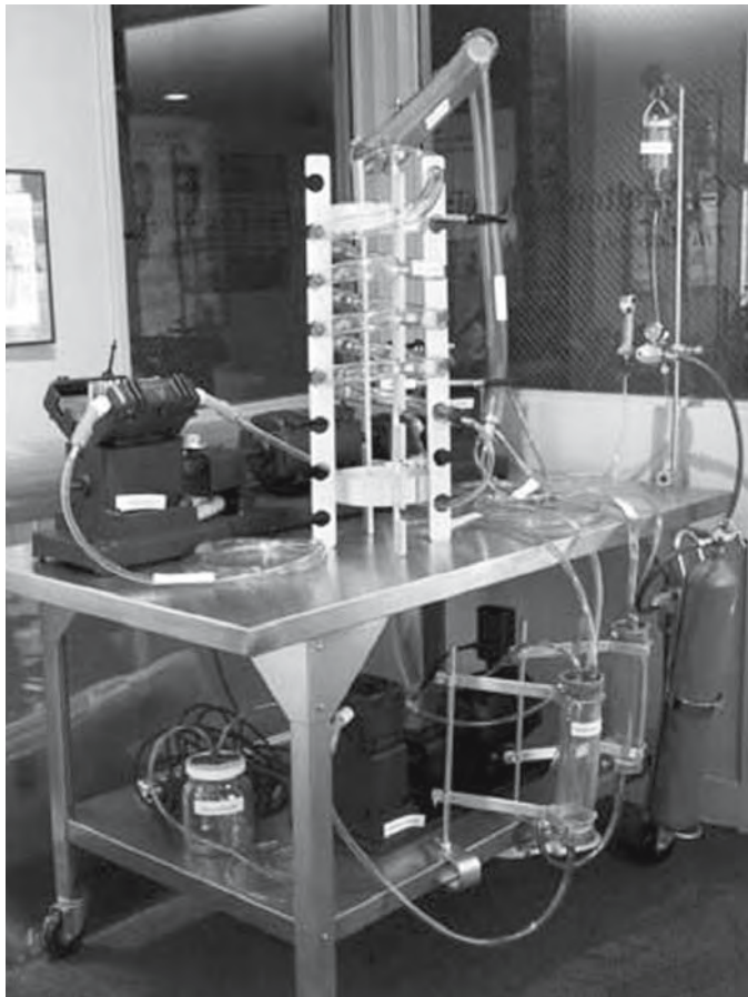
Fig. 2. Heart lung machine developed at the University of Minnesota by Dr. C. Walton Lillehei and Dr. Richard DeWall. Photo courtesy of Dr. Robert Gallegos.
