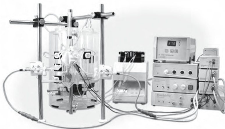
Fig. 1. ADInstruments Langendorff perfusion setup. Reprinted with permission from ADInstruments Inc. ( www.adinstruments.com ).
